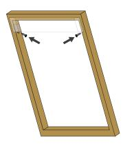
Step 3: Use one screw on each side to fix the cartridge in place.
