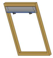
Step 2: Move the bar at the bottom of the fabric out of the way so you have clear access to the holes for the screws.
