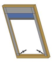
**Step 3**: Use the remaining two screws to secure the channels into place. Remember not to over tighten them.
