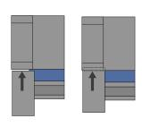
**Step 2**: Slot the channel into place just under the cartridge fascia (there is a small tab to guide the channel into place, the front of the channel should sit between the fascia and this tab)
