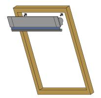
Step 1: Slot the cartridge into place at the top of the window.
