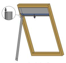
**Step 1**: Make sure that the handle is sitting centrally on the fabric, if it has moved then simply slide it sideways back into position (so an equal amount of fabric shows on both sides of the handle)Pull the blind down just far enough to be able to slide the fabric into the channel. The end of the channel has been angled outwards to allow the fabric to feed neatly into place.
