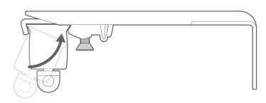
Rotate the headrail so that the back lip slots into the locking part of the bracket, then tighten the bracket screw to secure the rail in place.
