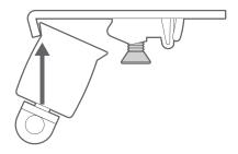
To do so, locate the front lip of the curtain headrail into the front hook of the bracket.
