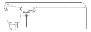
Tighten the locking screw in the bracket to lock the rail in place.
