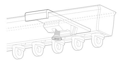
Clip the brackets onto the rail, spaced out as per page 1.
