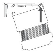
Situate the front lip of the headrail into the front of the bracket.
