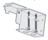
Where the brackets are screwed into the lintel (or 'ceiling' of the recess)
