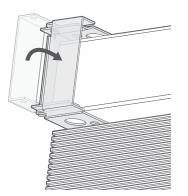
Lift the blind to the window and slot the headrail into the open brackets.
