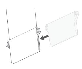
Slide the weight into the pocket at the bottom of the louvre.
