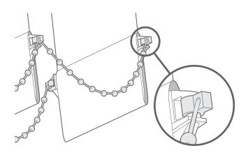
Clip the stabilising chain onto the weights, one chain will run along the back and the second will run along the front. Any excess clips can be cut away, just snip the cord flush to the last clip attached to a weight.
