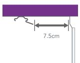
If you're using top-fix brackets, make sure that you mount them at least 7.5cm in front of either the window frame, or any protruding vents or handes, if there are any. This allows space for the louvres to turn open and closed.
