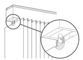
Hook the control wand onto the eyelet at the end of the hooks.
