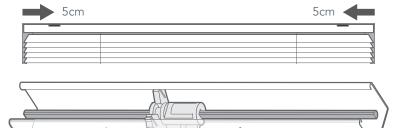
The outermost brackets should be mounted at least 5cm in from the ends of the blind.
