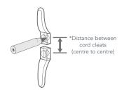
Mark the hole positions and drill as required. Use the screws provided to attach the safety cleat to the wall.
