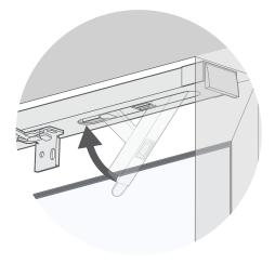
Hold the Click2Go™ rail up against the top of the recess, then push the lever firmly upwards until the rail snaps into place. If the rail is not quite tight enough then this can be easily adjusted:
