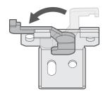
Hook the front lip of the headrail over the protruding hooks at the front of the bracket, then raise the back of the headrail so that it's level. Holding it in this position, swing the swing-arm over and press it firmly against the headrail to lock it in place.
