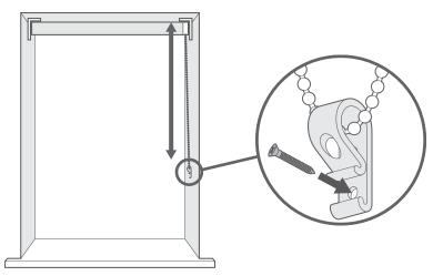
The cord retaining device must be installed at the maximum distance possible from the control mechanism to prevent looped cords from becoming slack.
