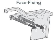
Where the brackets are screwed onto a facing surface (a wall or window frame)
