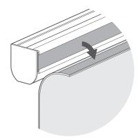
The fabric attaches at the front with velcro, simply peel the fabric away from the headrail.
