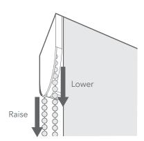
Pull down on the front part of the chain to lower the blind, and pull down on the rear part of the chain to raise the blind.
