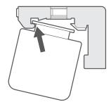
Situate the front lip of the headrail into the front of the bracket.
