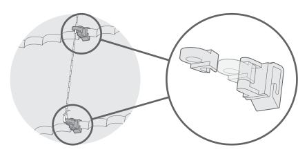
At the back, the cords attach to the fabric using clips, which double as a child-safety feature. These clips are in two parts, and can be easily unclipped to separate the cords from the fabric.
