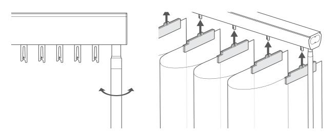
Twist the control wand to turn the hooks so that their 'open' part is facing into the room.
