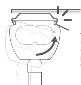
Then twist the back of the headrail upwards until it snaps into place in the rear hook of the bracket.
