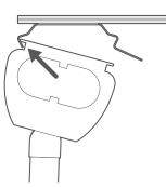
Rest the front lip of the headrail in the front lip of the bracket.
