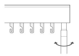
Twist the control wand to turn the hooks so that their 'open' part is facing into the room.
