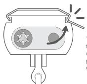
Then twist the back of the headrail upwards until it snaps into place in the rear hook of the bracket.
