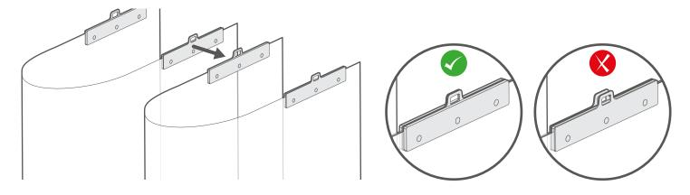
Hook the louvres onto the rail as shown, with each pair of hangers sharing a hook.
