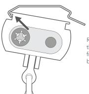
Rest the front lip of the headrail in the front lip of the bracket.
