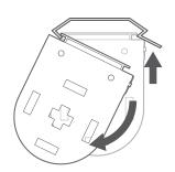
To release the blind from the brackets at any point after installing, push up firmly against the tab protruding from the back of the bracket. At the same time, twist the back of the headrail downwards to disengage it at the back.
