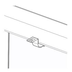
The brackets slide between the glass and the rubber seal.
