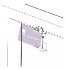
Slide the bracket into place so that it's lined up with the edge of the card. Do the same on each side, top and bottom.
