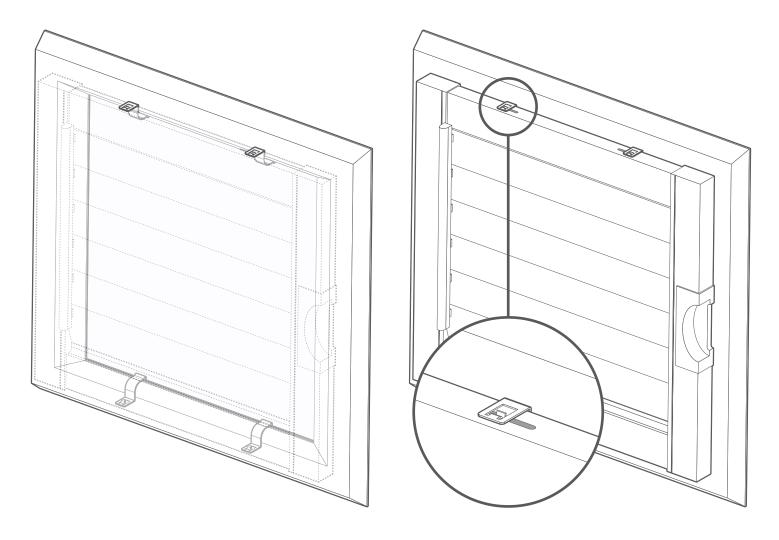
Line up the notches in the top and bottom frames of the Shutter with the brackets, and push the Shutter back against the window until it slots into place.
