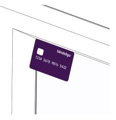
To correctly locate the brackets, take a standard sized debit or credit card and hold it in the corner of the glass.
