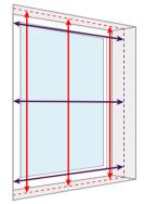
• Measure in 3 places for both the width and the drop, use the smallest measurement
