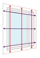
• To minimize light leakage we recommend that the Wave curtains overlap the window recess by at least 150mm at the top and on each side
