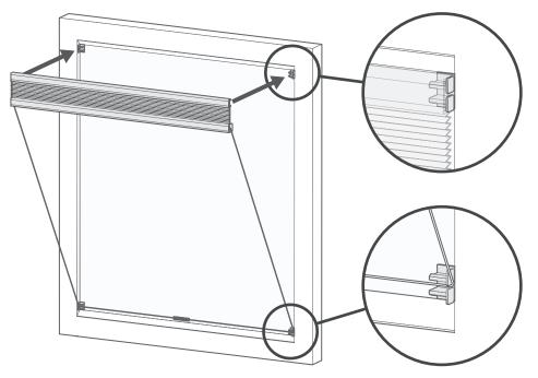
Clip the headrail onto the brackets at the top of the window by aligning the rail with the brackets and pushing the rail back towards the glass until you hear it click into place.
