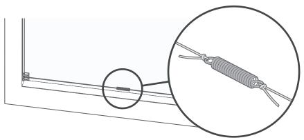
At the bottom of the blind the cord is connected to both ends of a small spring. Until the knot at one side of the spring.
