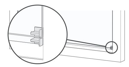
Slot the brackets back into the corners, as per step 1 of this guide.
