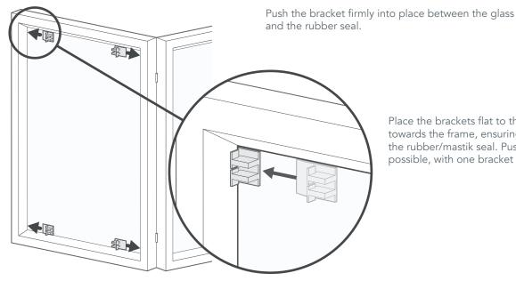
Place the brackets flat to the glass and push them in towards the frame, ensuring that they slide in under the rubber/mastik seal. Push in each bracket as far as possible, with one bracket in each corner of the glass.
